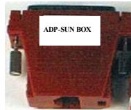
Part # ADP-SUN BOX SUN Workstation connector adaptor RJ45 socket/DB25 Male
